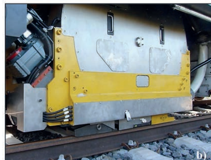
Fig. 1: Rotational planing – a new rail treatment technology. a) mode of action; b) Rotational planing unit; c) Rotational planing tools
