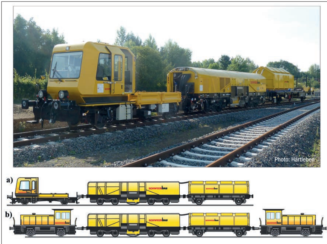
Fig. 2: Rotational planer D-HOB 2500 (in the middle), control module and chips module a) mainline version b) metro version
